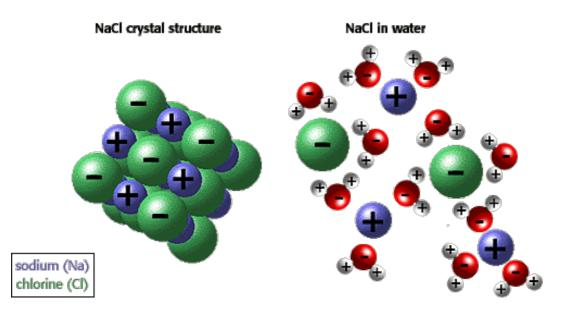
When we dissolve an ionic compound it is the separate ions in the compound being split apart and bonded to the water.
