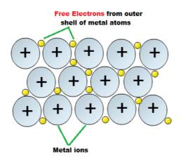
These are strongly bonded structures which have HIGH boiling and melting points.
